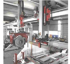
In a typical system wheels are transferred by gravity or by a gantry handling system onto a partially immersed roller drive system. The wheel is rotated as probes scan mechanically or electronically over the tread, boss and web areas. Any defects detected cause the wheels to be marked and removed from the manufacturing line. The cycle time can be less than 1 minute.
