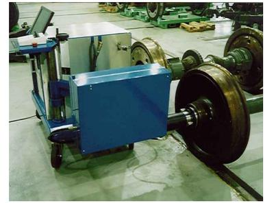
These are mobile units used in maintenance workshops for periodic inspection of axles for fatigue cracks and other defects on both exposed and hidden surfaces. The unit is connected to each axle in turn and a rotating probe head travels down the bore. The inspection is completely automatic and produces an image displaying any defects above a preset threshold.
