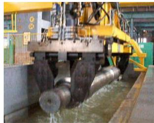
Ultrasonic immersion tank with adjustable roller drives for axle testing (left) integrated into conveyor and gantry handling line
