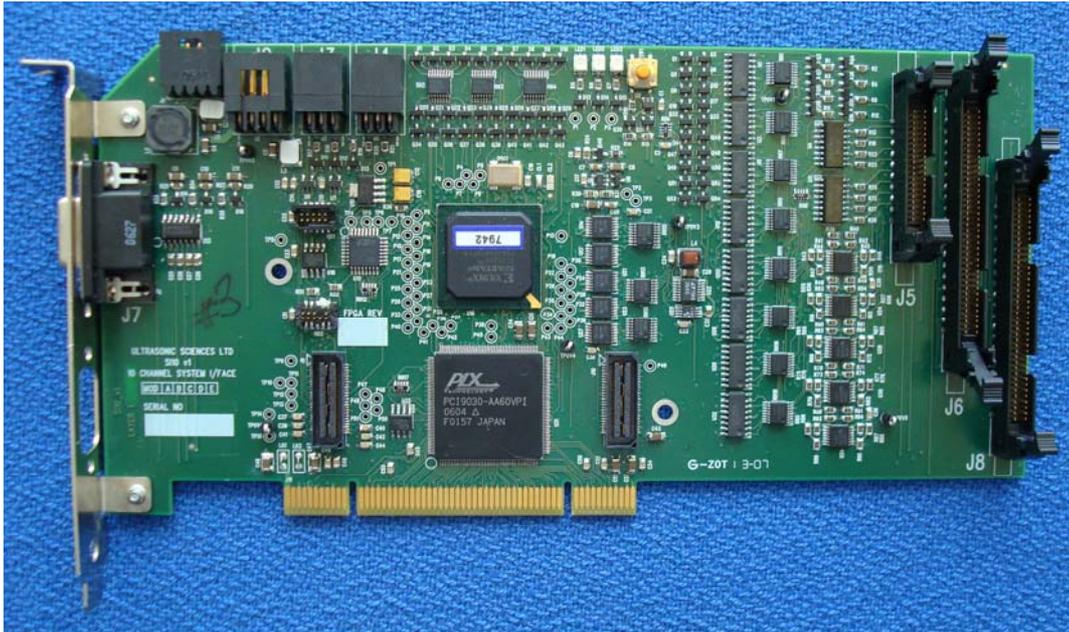
10 axis motion control for DC servo and stepper motors
